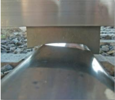
Initial rail condition (damaged, worn)
